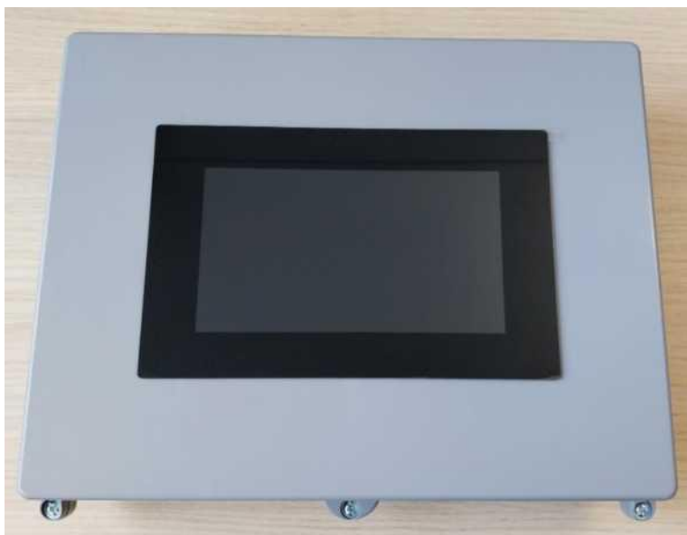
Figure 7: Control center including display
